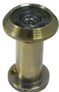
MODEL: DV10 Zinc alloy viewer Size: \Phi 12\text{mm} , 14mm, 16mm Door thickness: 35-55mm, 60-100mm 180° 200° Finish: PB. AB. AC. CP. SN. Synthetic Resin Lens
