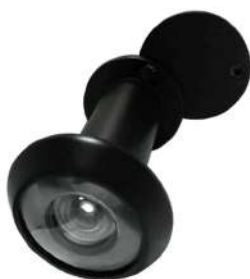
MODEL: DV08 Brass door viewer Size: \Phi 12\text{mm} , 14mm, 16mm Door thickness: 35-55mm, 60-100mm 180° 200° Finish: PB. AB. AC. CP. SN. Synthetic Resin Lens
