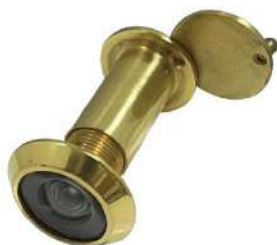
MODEL: DV04 Brass door viewer Size: \Phi 12\text{mm} , 14mm, 16mm Door thickness: 35-55mm, 60-100mm 180° 200° Finish: PB. AB. AC. CP. SN. Synthetic Resin Lens With Cover
