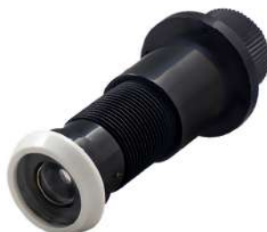
MODEL: DV12 Door Viewer Material: ABS/plastic Cover material: Synthetic resin lens with cover Finish: BN Diameter : 28mm Door Thickness: 35-55mm Viewing angle: 200 degree
