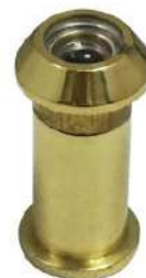
MODEL: DV06 Brass door viewer Size: \Phi 12\text{mm} , 14mm, 16mm Door thickness: 35-55mm, 60-100mm 180° 200° Finish: PB. AB. AC. CP. SN. Synthetic Resin Lens
