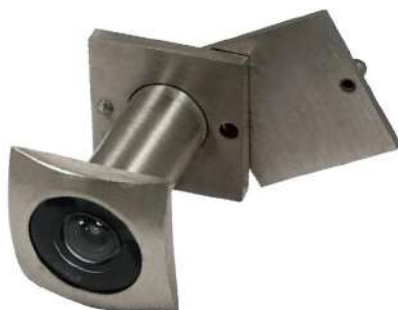
MODEL: DV11 Door Viewer Material: Brass Diameter size: 12mm, 14mm, 16mm Door thickness : 35-55mm Viewing angle: 180 degree/200 degree Finish: PB. AB. AC. CP. SN
